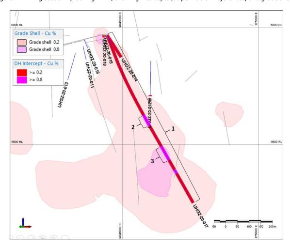
Figure 4: Drilling Section B, looking N-NE, showing intercepts (as per Table 2 references) and grade shells.
