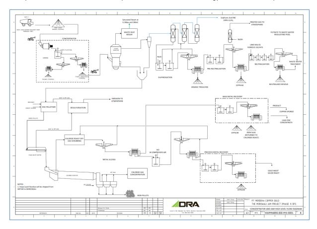
Figure 6: AIM Project High Level Block Flow Diagram
