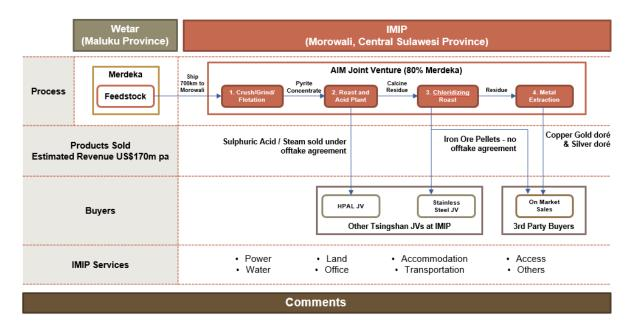
Figure 7: AIM Project High Level Block Flow Diagram
