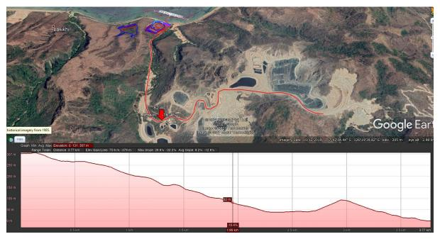
Figure 4: Satellite Image of Haulage from Wetar Heap Leach Pads to Barge Jetty
