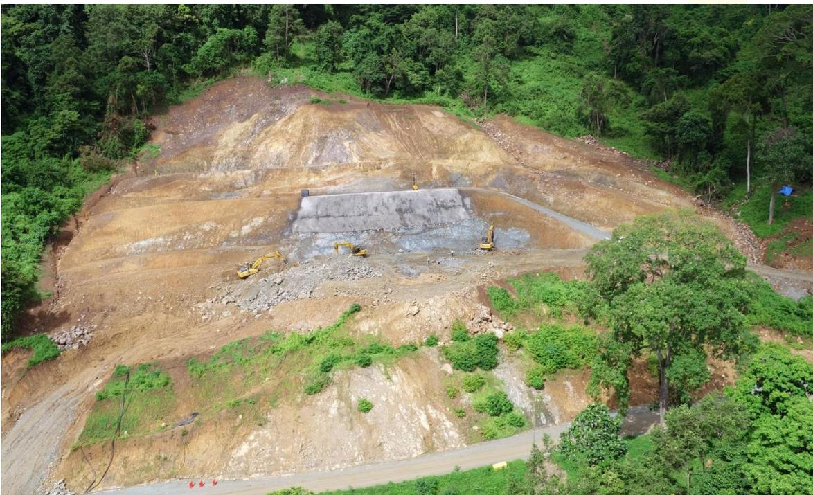
Figure 5 – Pit A sediment sump
