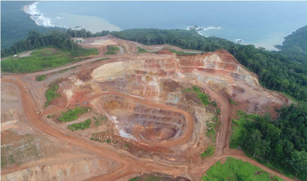
Figure 2 – Aerial view of the Heap Leach Pad showing 2 complete lifts with Lift 3 just starting
