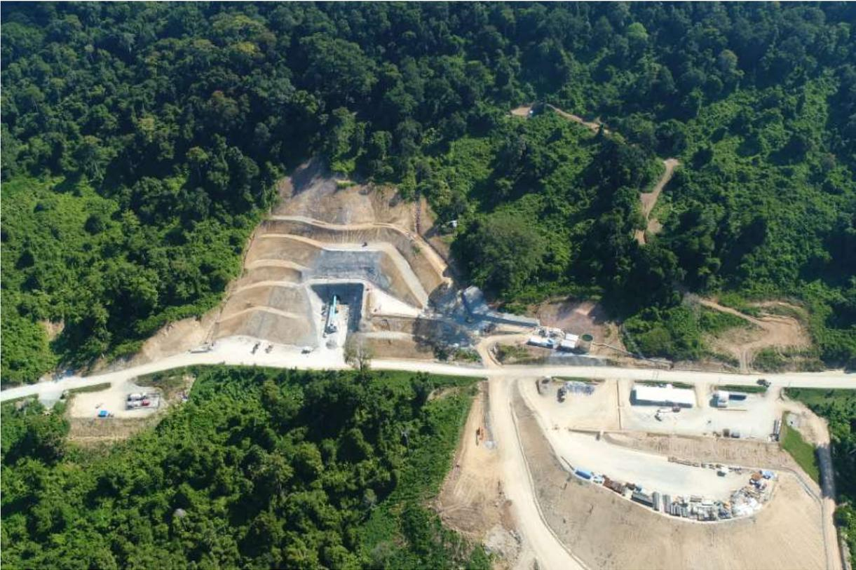
Figure 7 – OPP 2 Bulk Earthworks, slope stabilization and micropiles commencing.
