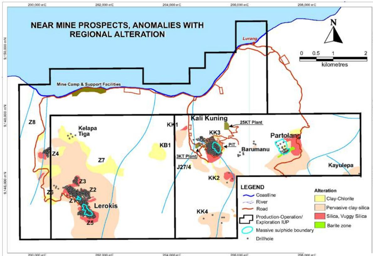
At Partolang, the program includes 4,000 to 5,000 m of reverse circulation and 650 m of diamond drilling. The main objective of this work is to complete initial step-out drilling over interpreted massive sulphide mineralisation, which is associated with an electromagnetic (EM) conductor. Drilling will be completed on a nominal 50 m spacing (initially). A secondary objective will be to evaluate the gold-silver potential of the overlying barite zone.
