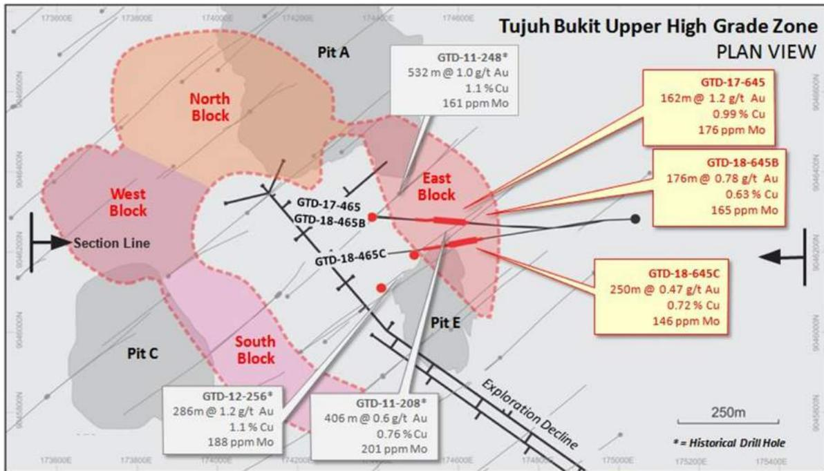
Figure 2 shows a cross section looking due north at the completed directional drilling program targeting the East Block of the Upper High Grade Zone.
