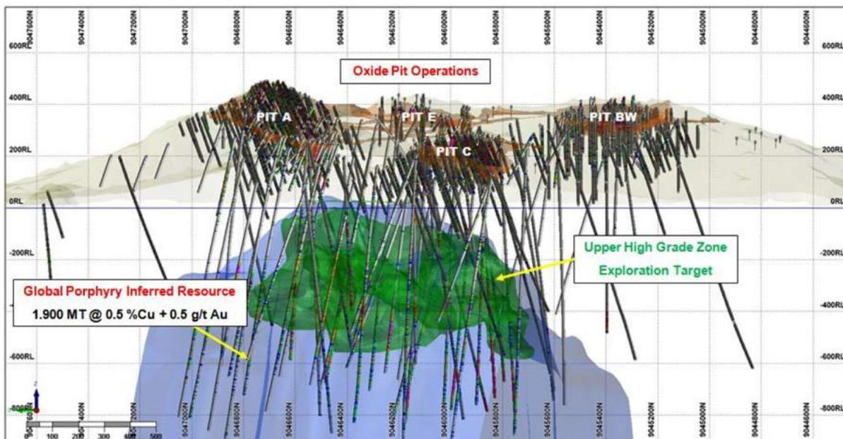
A Concept Study has been completed to analyse options to develop a bulk underground mine to exploit the UHGZ. This study identified a preferred scenario whereby four discrete blocks arranged around the relatively un-mineralised core will be developed sequentially as a series of block cave mines. All blocks have a common extraction level at minus 500 level with ore transported to a central common crusher.
