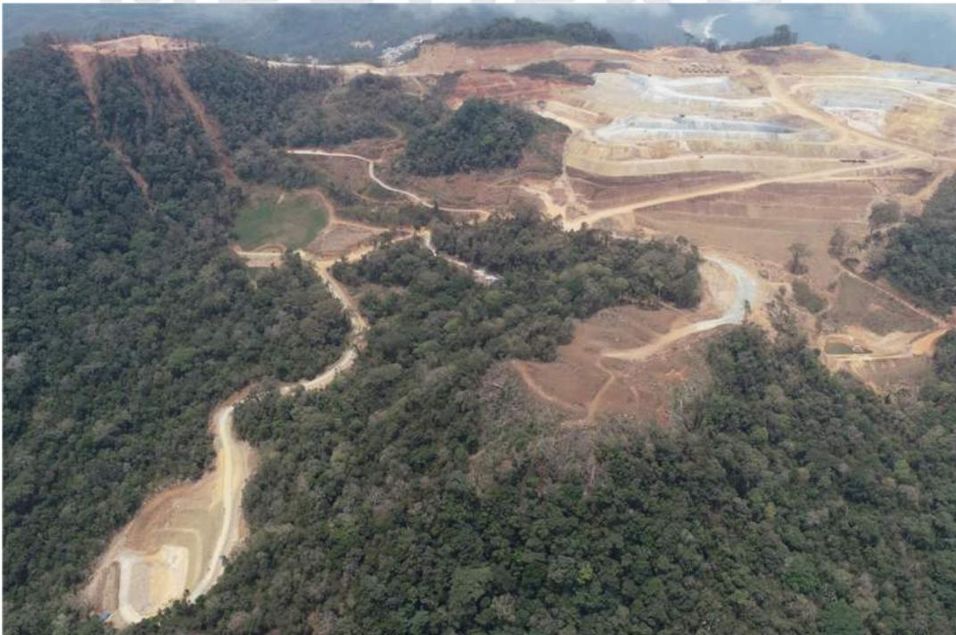
Figure 5 – Aerial view of the Heap Leach Pad completed lift 1 expansion and lift 4 continuing
