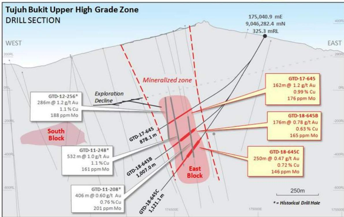
Figure 3 shows a more detailed cross section looking due north at the completed directional drilling program and the location of metallurgical composites with corresponding drill core assay results.
