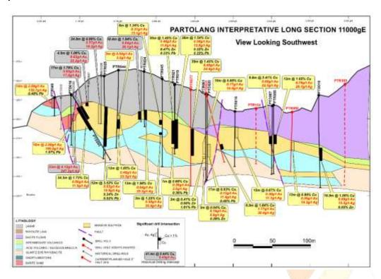
Figure 5 - Geological long section 11100gE, showing main geological zones, new drill traces (completed and proposed) with geology and significant new Cu/Au intercepts (where available)
