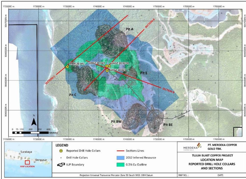
Hydrogeology drill hole MBH-20-041 was drilled as part of the PFS, including packer testing and piezometer installation. The hole was drilled outside of the known 0.5% Cu envelope to a depth of 792.5m as shown in Figure 4, and has subsequently extended this grade shell by returning a result of 368m @ 0.5 % Cu and 0.5 g/t Au.
