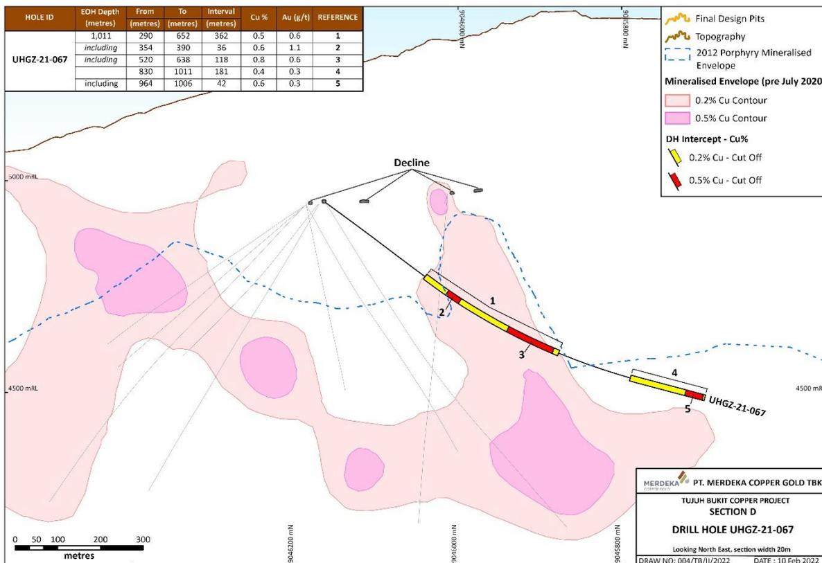
Figure 5: Drill section D, showing drill hole UHGZ-21-067 intercepting two mineralised envelopes and drilling intercept information.
