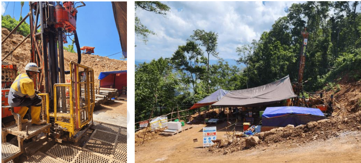
Figure 14: Diamond drilling along strike of Pit A
