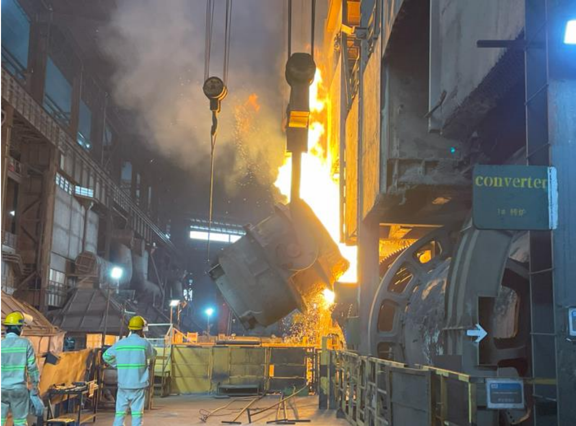
High Grade Nickel Matte Converter (HNMI)
