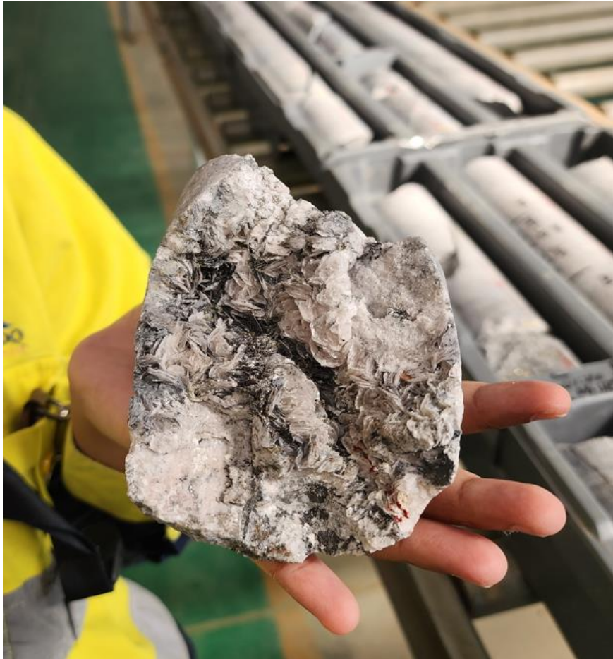
Figure 8: Coarse blades of alunitic crystals in the drill core
