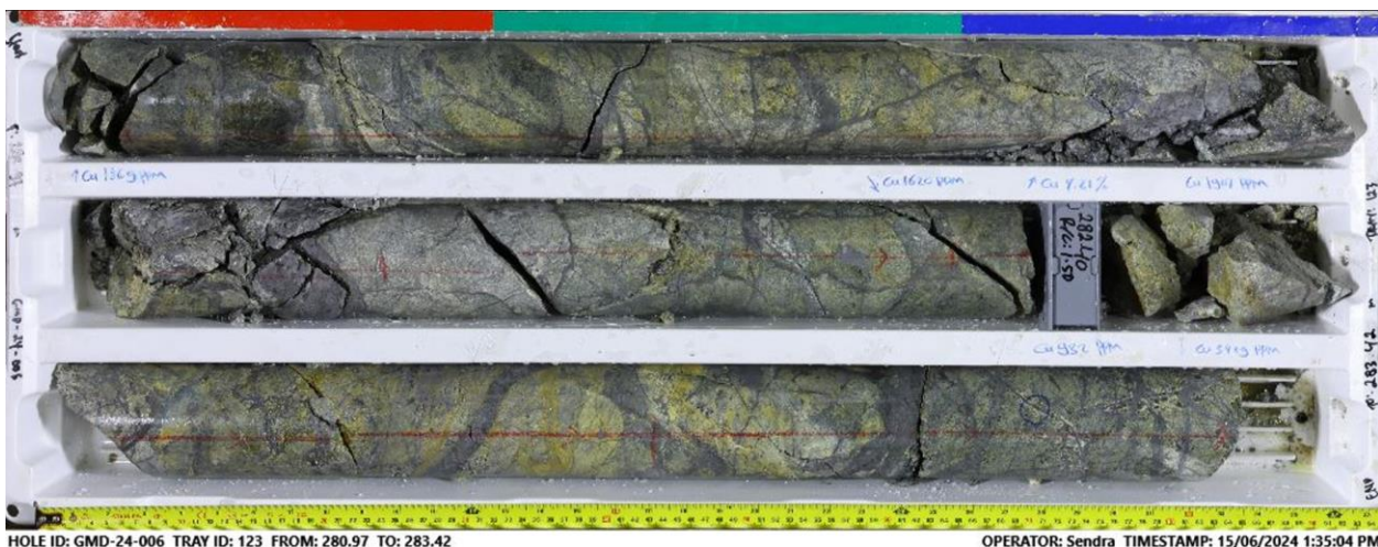
Figure 6: Gua Macan drill core from GMD-24-006 showing porphyry style stockwork quartz-magnetite-chalcopryrite veins
