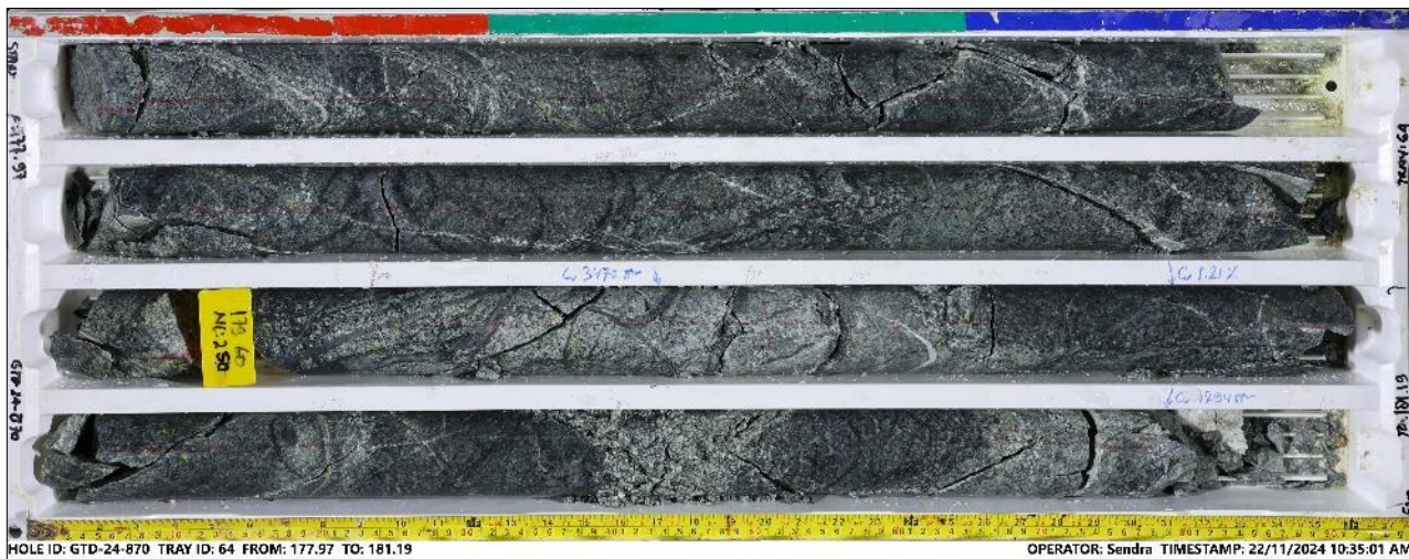
Figure 10: TB North drill core from GTD-24-870 showing porphyry style stockwork quartz-magnetite-chalcopyrite veins
